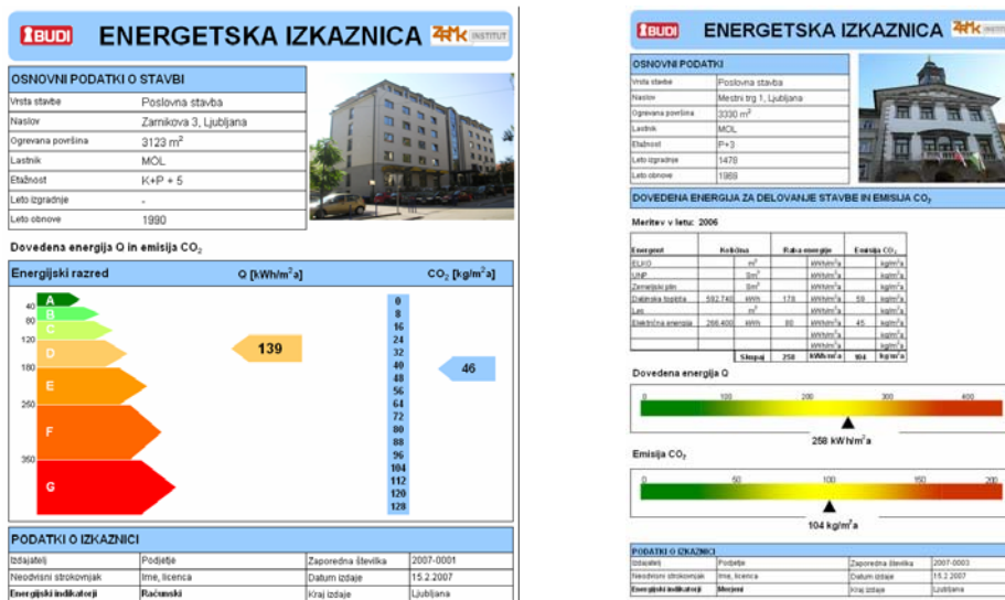
Figure BUDI calculated energy certificate (for all buildings, but primarily for existing residential) and metered energy certificate (existing non-residential), used as proposal for regulation.
